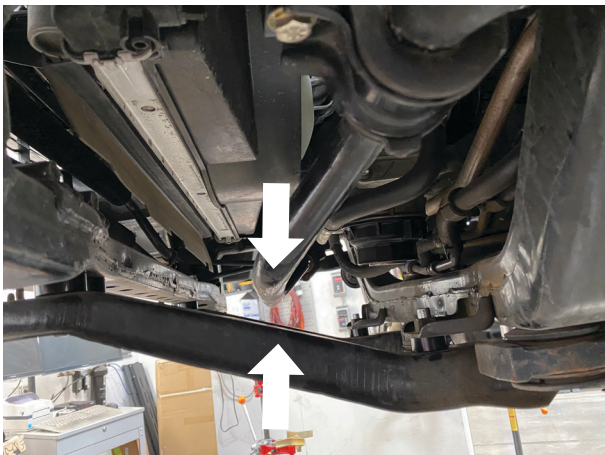
Fig. 16: Check clearance of the sway bar.
