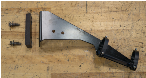
Fig. 12: Reservoir bracket assembly.
