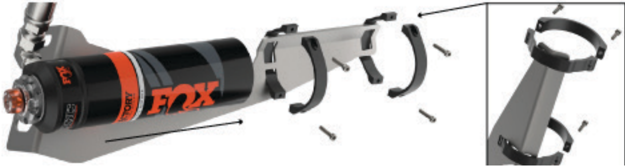
Fig. 10: Diagram of reservoir and bracket interface.
