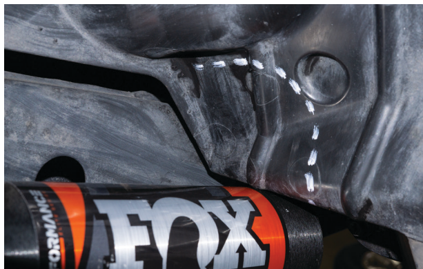
Fig. 25: Cut the fender liner.
