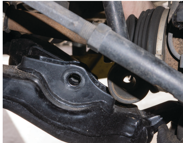
Fig. 5: Remove the bolt from the lower control arm.
