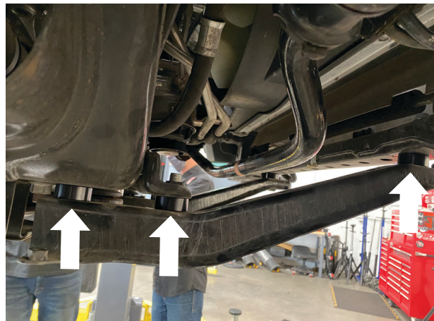
Fig. 17: Install the skid plate spacers
