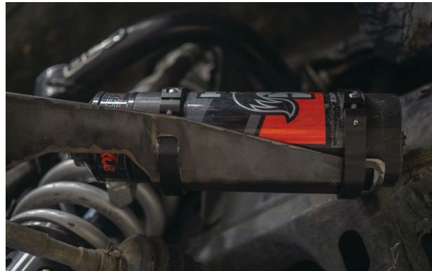
Fig. 8: Locate the clamps accordingly.
