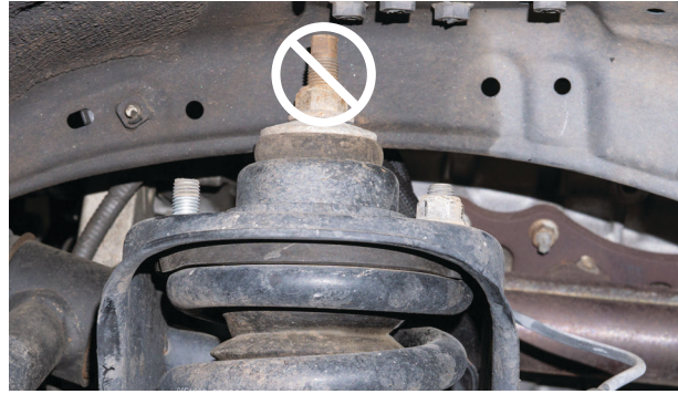
Fig. 4: Remove the three top hat nuts.
