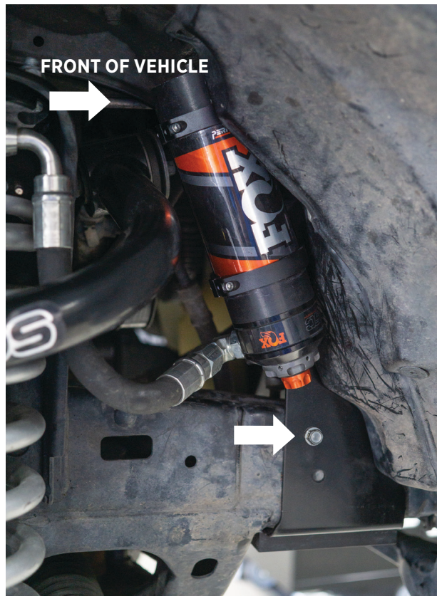
Fig. 13: Install the self tapping screw into the existing hole.
