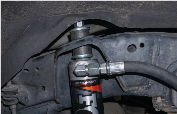
Fig. 23: Install the stem top nut (driver side shown).
