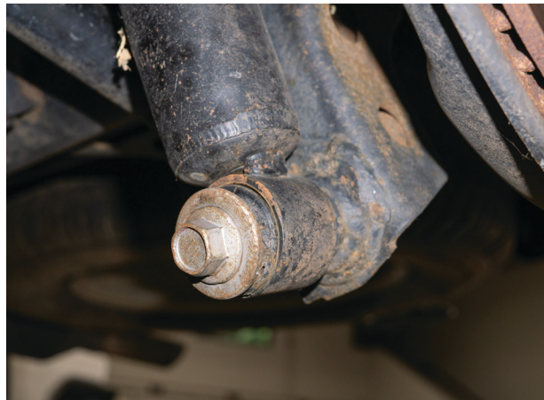
Fig. 21: Remove lower shock mount bolt.
