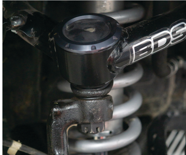
Fig. 7: Reattach UCA to the upright.
