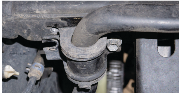
Fig. 11: Remove sway bar bracket.
