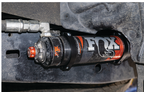
Fig. 26: Mount the reservoir to the bracket (driver side shown).
