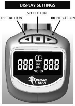
The display features Low and High pressure alarms. The display is supplied with the Low pressure alarm set at 5psi and the High pressure alarm set at 30psi. These pressure alarms can be set for your application.
