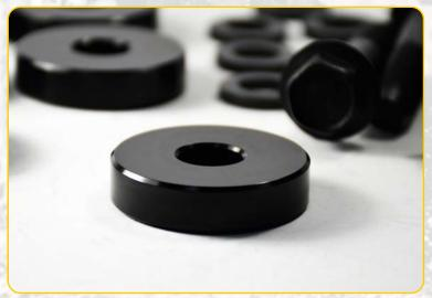
CNC machined billet aluminium (6061) 12mm K-frame spacers to suit Nissan Patrol Y62. Black anodised for discreet installation.
