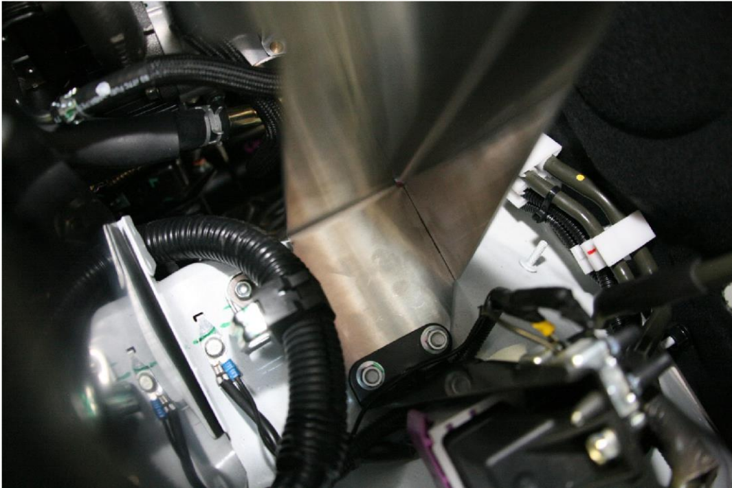
mounting bracket installed
