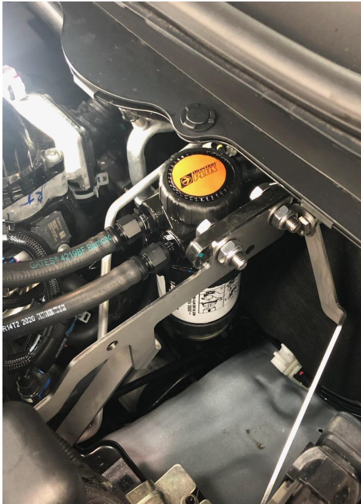
Completed installation of the Fuel Manager PRE-FILTER FM664DPK
