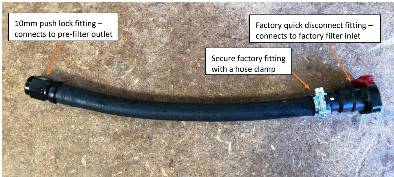
hose construction from pre-filter outlet to factory filter inlet
