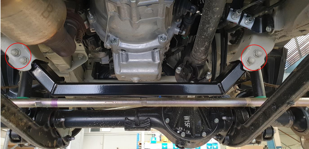
Figure 1. Shows CB297 installed. 4 bolts circled.
