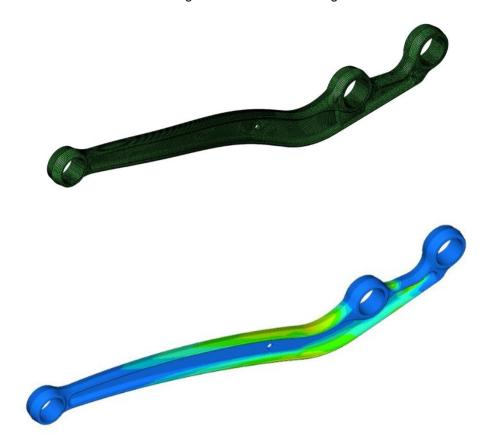
Figure 2: Radius Arm Mesh and Stress Contour
