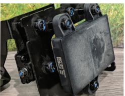
The sensor is attached to two brackets. These need to be removed. This is done by poping off ball joint clips using small lever. Ensure you are gentle with sensor
