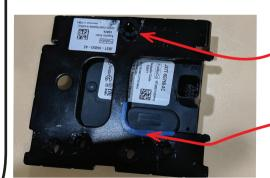
Drill holes to 12mm after removing pins. then insert clips.
