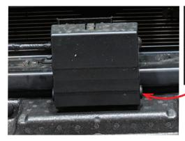
Remove the cover by taking out the two plastic clips.
