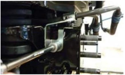
3. Relocate cooler pipe higher as per photo so that winch cradle can be located into position
