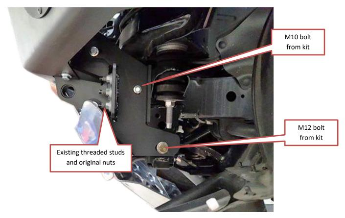
6. Locate and fasten light mounting bar using supplied M10 bolts into top of bar
