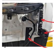
Remove plastic facia clips by drilling out pop rivets and removing nuts.
