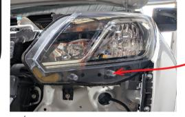
Trim the lugs off lower light with multi tool ensuring minimal dust entry.
