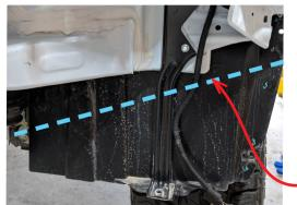
Trim plastic wheel arch liner from bottom of chassis at a straight line leaving 1cm between line and body here.
