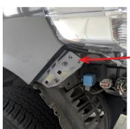
**b.** Remove plastic bracket on leading edge of guards. Ensure you replace head light bracket bolt.
