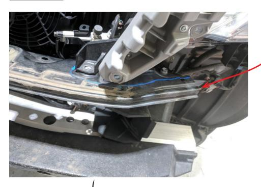
Remove long bracket and replace with Rhino LC200 head light mounting brackets included in the box
