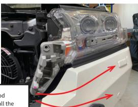
Now is a good time to install the parking sensors and headlight washers if fitted. Blanking plugs for these will be supplied if needed on your model.
