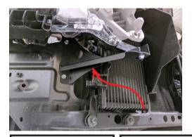
Remove two m6 bolts from the firewall and mount the headlight support brackets on the drivers and passenger side of the vehicle.
