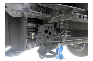
**a.** Remove Facia and alloy bumper beam. Remove front chassis brackets keeping nuts for use on installing Rhino chassis brackets.
