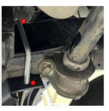
If not previously complete install sensor housing directly into wing.
