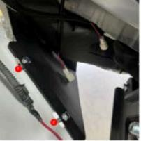
Install Bash Plates using original bolts and CSK bolts provided.
