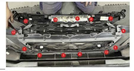
A-28 Detach chrome trim from grill assembly by removing screws.
