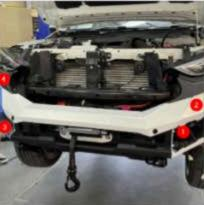
Install wiring loom and insert sensors into original positions.
