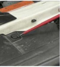
Remove clips for retaining grill assembly.
