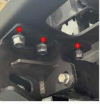
Use provided U-Shaped bolts to secure wing support bracket.
