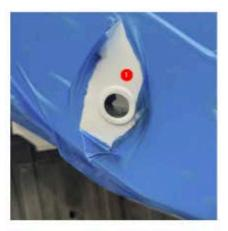
A-27 Detach grill assembly by removing screws and releasing clips around the perimeter shown.
