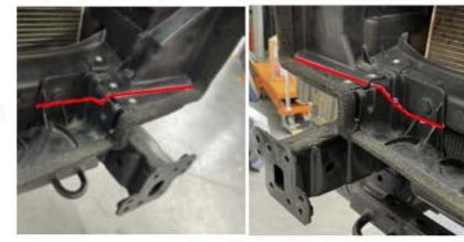
A-18 Trim off sections marked in previous step. Remove and discard the sections that come free.
