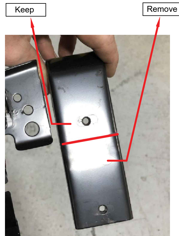
Figure 6: First member that requires cutting
