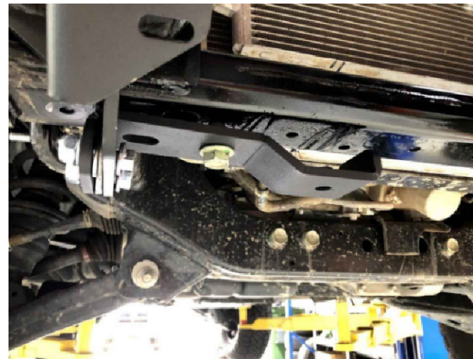
Figure 8: Painted surface after removing recovery point
