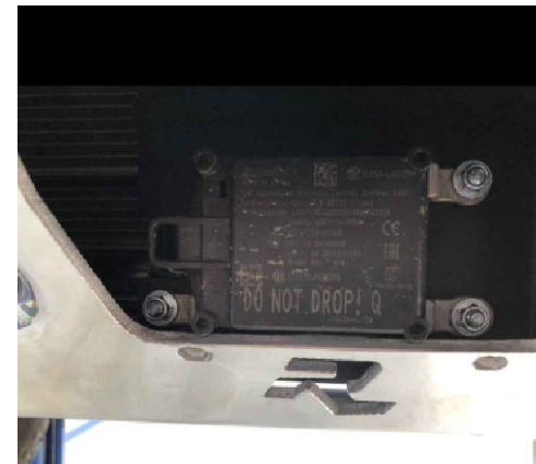
Figure 25: Front view of radar bracket
