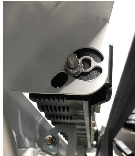
Figure 20: Mounting the light bar
