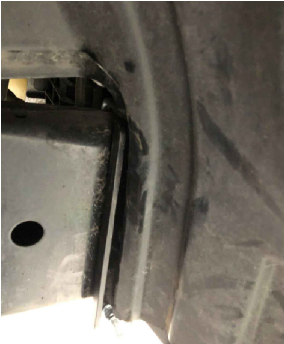
Figure 36: Trimming the wheel arch liners.
