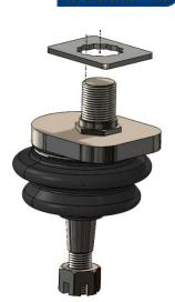
The ball joint can be rotated through 12 fixed positions by re-positioning the hex on the ball joint into the doublehex washer, as shown to the right.
