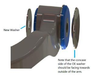
Unlike bonded or rubber bushings, SuperPro bushings pivot freely and so can be torqued at full droop.
