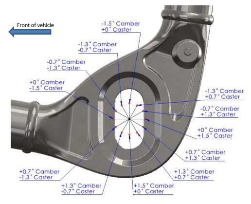
In conjunction with rotating the ball joint, the ball joint can slide in and out in the slot, which allows for +/- 1.5 degrees of additional camber adjustment.
