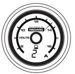
**Background Colour** *Mode / Beeps:* 2 Selections: 13 colours Press and hold to select the programming button to select the colour that the gauge backlight will display during normal operation. There are 13 different colour options.
