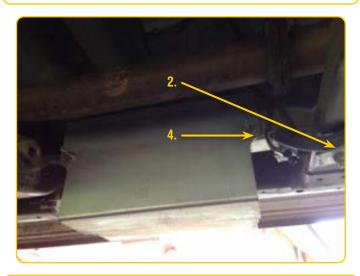
3. There are two holes in the back of the box. Place 2 x 6mm long bolts through holes. One bolt sits on top of the chassis and one under the chassis rail. Place bracket onto bolts. Place nuts on and tighten.
