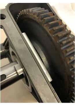
Be certain that the circlip is correctly fastened and that the bronze bush and oil seal are correctly re-fitted, and re-fit the brake assembly to the mainshaft. If the winch had the three spring disc washers behind the circlip, then re-fit these, and then fit the mainshaft end cap with the M12 schnorr washer and Cap Head bolt. Ensure that the bolt is tight.
