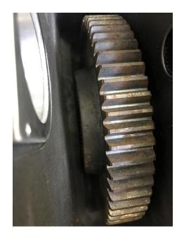
Now slide the large cam gear over the mainshaft and insert the mainshaft, taking care to fit the large intermediate gear, round shim and circlip.
